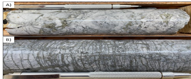
A) EMR22-020 at 162 m: Brecciation of silicified feldspar porphyry with quartz-pyrite cement. B) EMR22-020 at 168 m: Cluster of pyrite-quartz veinlets cutting clasts and cement of breccia, note sulfides up to 15%.
