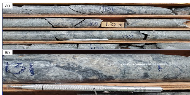
EMR22-019 at 130.5 to 134.5 m A) Quartz cemented breccia; dark gray-black veinlets are made up of quartz and 30 – 40 % very fine-grained pyrite. B) Close-up photograph showing later phase of brecciation from dark quartz-pyrite veinlets.
